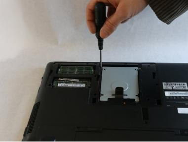
• Locate the gray hard drive cover, and remove the four corner 3.5mm screws.
