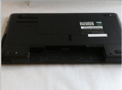
Completely remove the battery from the laptop.
