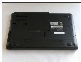
Unscrew the 4mm screw, and slide the cover off away from the computer to reveal the housing for the hard drive and RAM boards.
