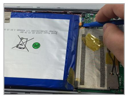
Free the battery from the motherboard by prying slightly with the opening tool.
