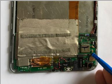
Using a plastic opening tool, pry the black wire connectors pointed to in the picture.
