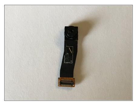
The front camera should be out of its compartment by now. Reinstall the new camera.
