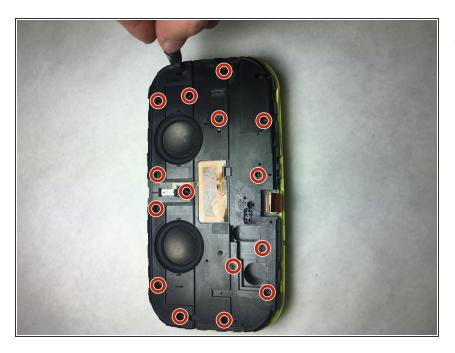
Unscrew fifteen 6.2mm Phillips #0 screws and lift the black plastic plate from the case.
