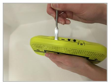
With plastic spudger wedge in between the top and bottom casings to force sepearation. Exposing the inside components of the Republic Deck.
