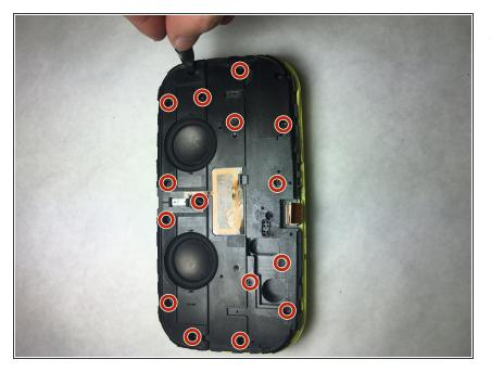
Unscrew 15 6.15 mm Phillips #0 screws and lift the black plastic plate from the case.
