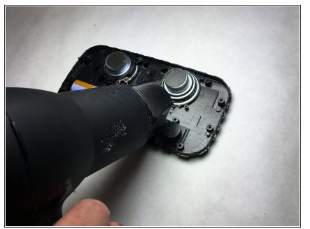
Use the hairdryer to soften the glue holding the speaker to the plastic plate.
