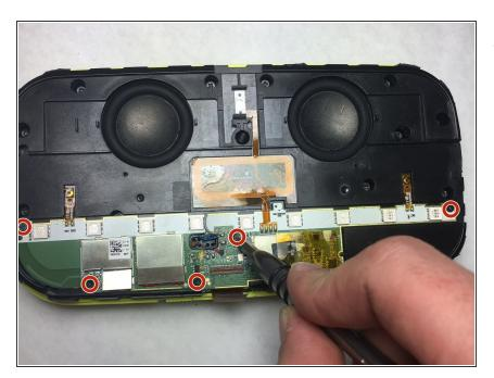
Unscrew 5 3.63 mm Phillips #0 screws securing the circuit board.
