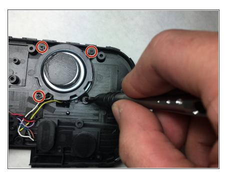
Remove 4 3.63 mm Phillips #0 screws holding the bracket.
