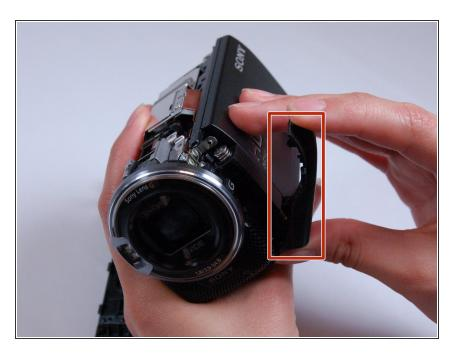
Carefully pop off the casing strip on the camera's left-hand side near the lens.
