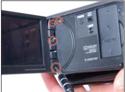
• Use the Phillips #00 head to remove the following 5.5mm screws on the left-hand side.
