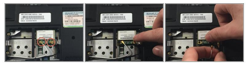
• Unplug the two connecting cables by lifting them up. They should unclip easily.
