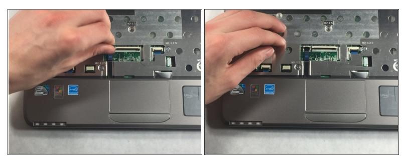
• Lift the small black clip and remove the ribbon cable before proceeding.
