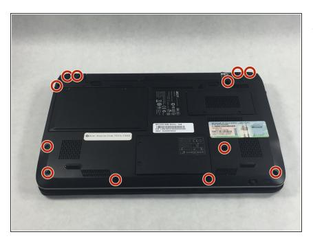
Use the screwdriver to remove all the Phillips #00 (M2-L2.5 mm) screws shown here.
