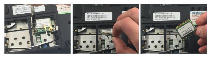
• Remove the screw Phillips #0 (M2-L3 mm) holding down the network card. Pull out the card.
