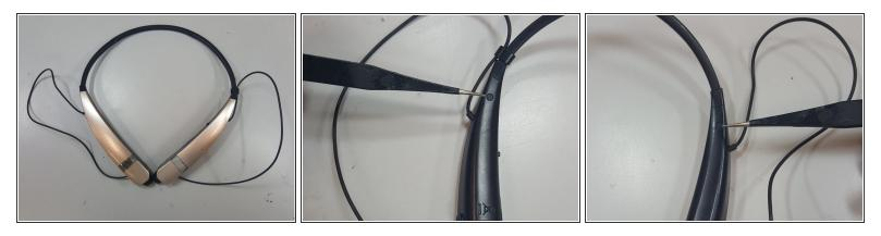
Locate the right and left side speaker where the hidden screw is located and remove the rubber piece covering the screw.
