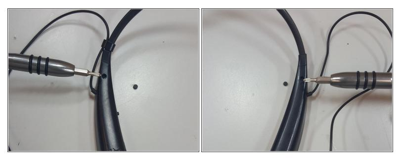
• Using a Philips #00 screwdriver, remove the hidden screws from both sides.
