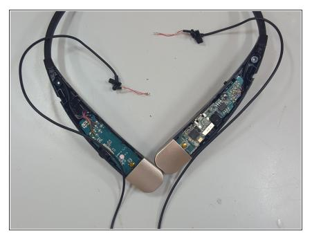
• Once the speakers have been desoldered, replace with new ones.
