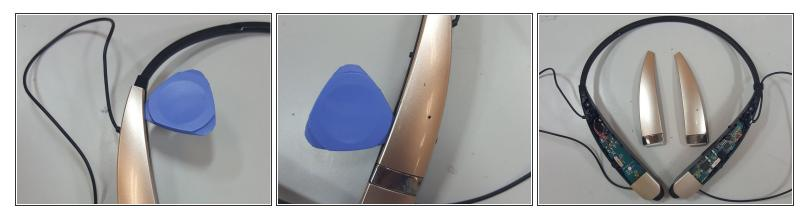
Use a guitar pick or any opening tool to pry open the housing for the side you want to replace the speaker.
