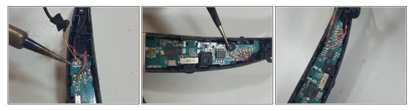
• Right side can be de-soldered right away but the left side speaker solder connection to the board is covered by rubber material which needs to be removed first before it can be de-soldered.
