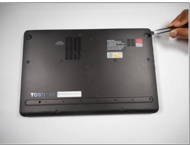
Remove the 9 rubber gripper pads on the back panel of the laptop using tweezers.
