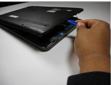
Take off the back panel open by sticking the plastic opening tool into the seam of the laptop, and pushing the opening tool downwards.
