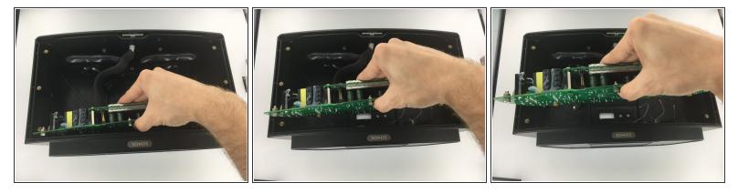
Remove circuit board by lifting it straight away from the rear plate.
