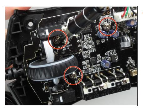
Use a Phillips #0 screwdriver to remove three 5.5 mm screws.
