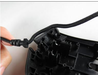
Remove the USB cable by pulling it up and out.
