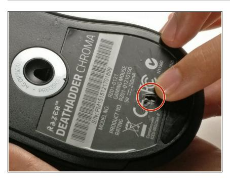
Use your fingers to identify the location of the screw under the bottom label.
