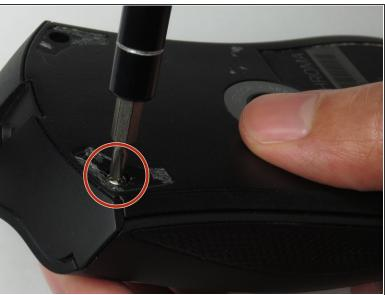
Use a Phillips #0 screwdriver to remove two 6.7 mm screws.
