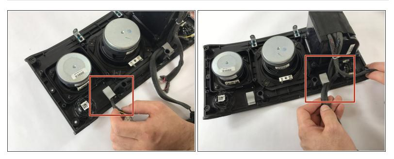
• Remove the wires from the plastic clips on the bottom of the front panel.
