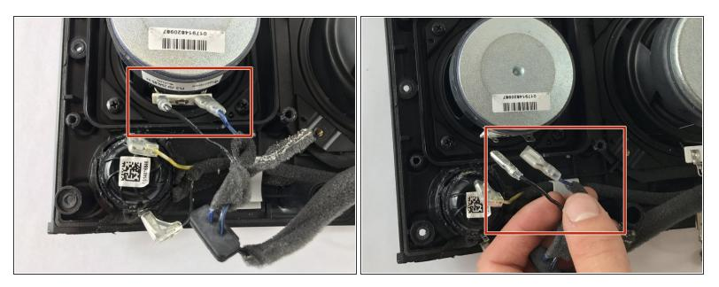
• Unplug the wires connected to the left speaker.
