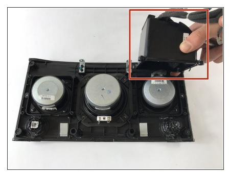
• Remove the plastic speaker cover by lifting up and away.
