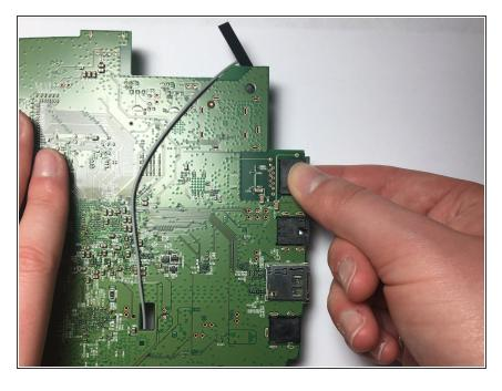
Using your thumb and pointer finger, carefully pinch the Ethernet port and pull it to the right, away from the motherboard, to remove it.
