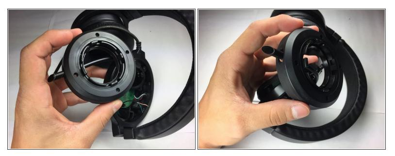
• Slide the speaker case laterally along the length of the microphone until the casing is completely detached from the headset.
