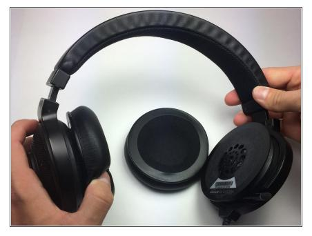
Continue sliding downwards around all edges of the ear cushion until the cushion is fully removed.
