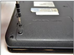
• Use a J00 bit to unscrew the single 4mm screw that holds the hard drive cover in place.
