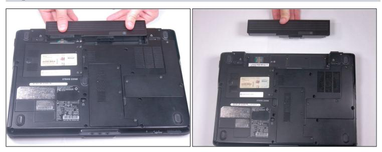
• Push the battery forward to eject it from the laptop.
