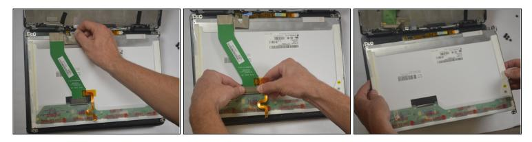
• Unplug the two cables connected to the screen.
