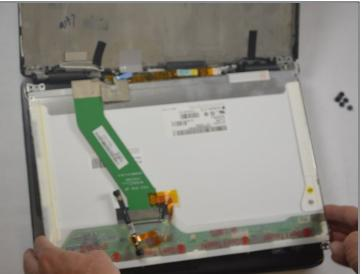
• Carefully remove the screen from the back cover.
