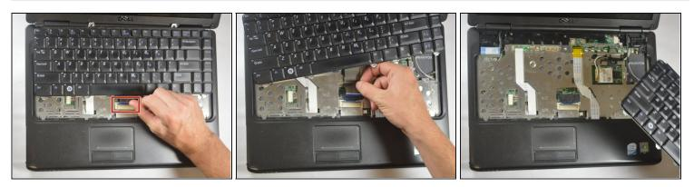
• Carefully lift up the blue latch on the keyboard cable connector and slide the cable out.
