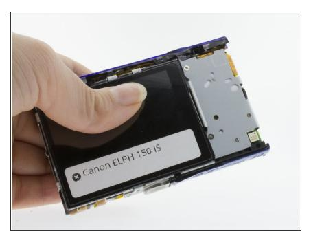
In order to replace the door, you must first remove the back plate off the camera. <u>Use this guide to do so</u>.
