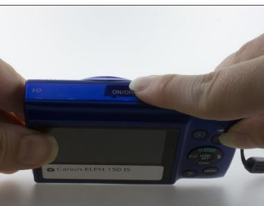
Safety First: Power down your camera by locating the ON/Off button on the top of the camera and holding it down until the screen and all lights on the camera go dark.
