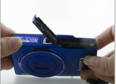
With the backplate removed, turn the camera so that the CARD/BATT. OPEN door is face up and to the right. Press down on the door as you slide it to the right. You should hear a click which indicates that the door is unlocked and will freely open.
