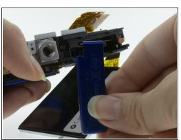
• With the CARD/BATT. OPEN door open, and the backplate off, gently pull the door from a 90 degree angle back towards you. Once you hear a pop (a sign that one side pin has released), you can slide the door away from you to release the pin on the other side as well. Remove door.
