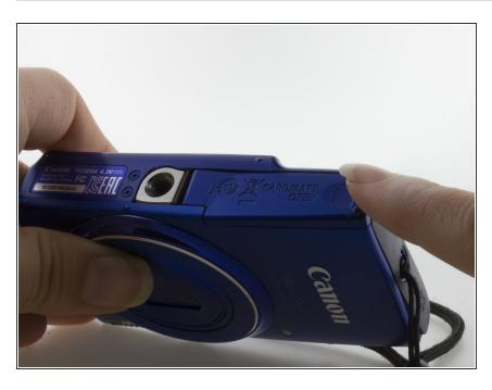
Locate the CARD/BATT. OPEN door on the bottom right of the camera.
