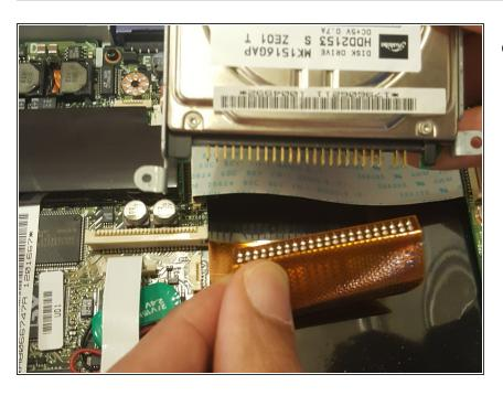
Remove the ribbon cable connecting the motherboard to the hard drive by pulling the female connector off of the pins attached the hard drive.
