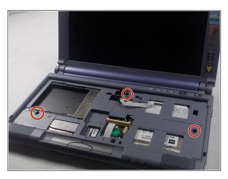
Remove the three 10 mm screws holding the casing to the top of the motherboard using a Phillips screwdriver.
