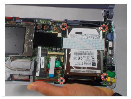
Remove the four 5 mm screws holding the hard drive to the motherboard.
