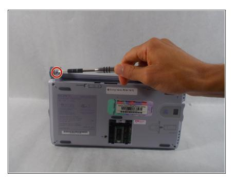
Turn the device upside down and remove the other 6 mm screw holding the casing to the device using a phillips head screwdriver.
