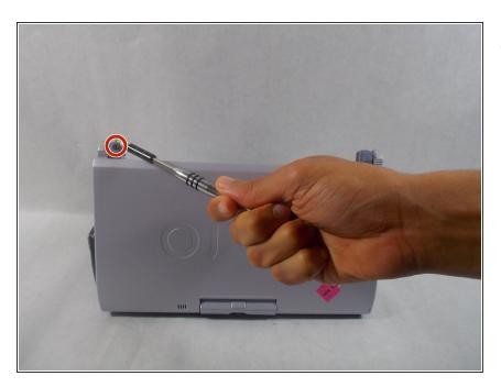
Remove the 6 mm screw on the left side of the battery that holds the casing to the device using a phillips head screwdriver.
