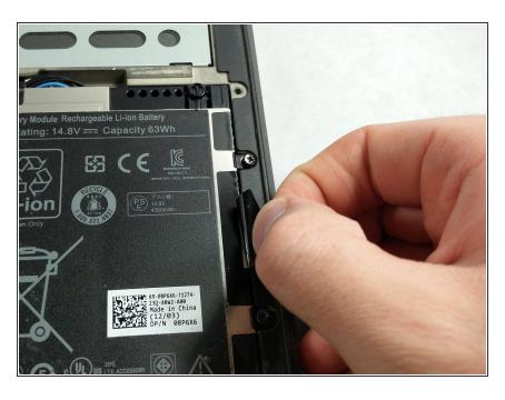
Now, remove the battery by gently pulling on the tab located between the two screws. The battery will pivot, and you will be able to completely detach the battery from the device.
