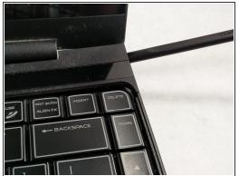
Now, flip the computer back over. Above the "DELETE" key on the edge of the computer is a small indent. Here you will use the spudger to pry this plastic piece up.
