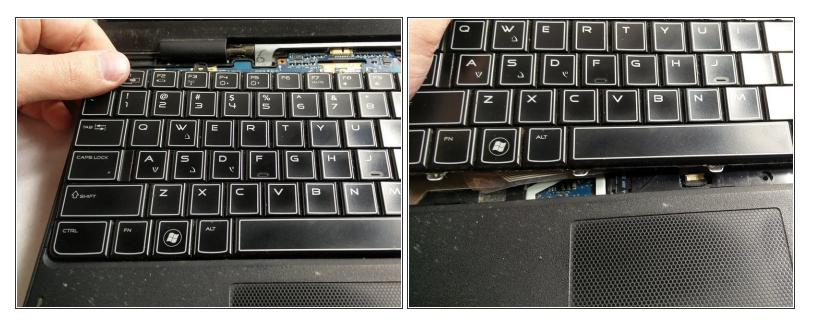
With both screws removed, gently lift up on the keyboard, and slide it towards the monitor. It will come out.
