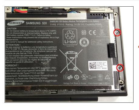
Unscrew the two circled screws holding the battery in place. These screws have retaining washers, so
