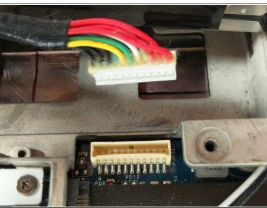
Next, unplug the battery cable (PD12) from the motherboard by gently pulling up.
