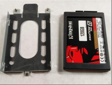
On both sides of the cage, there are two screws you have to unscrew to be able to remove the SSD.
