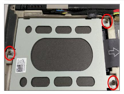
Remove the three screws attaching the hard drive tray to the laptop.
