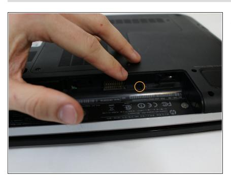
Move the switch in the battery compartment.
