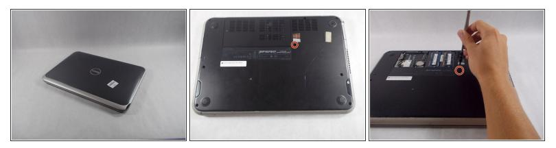
• First flip the device over, so the bottom is facing you. Then you will remove the highlighted screw.
