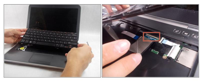
The ribbon connector seen in yellow can be removed by flipping up the plastic hinge clamp with a thin plastic pry lever
