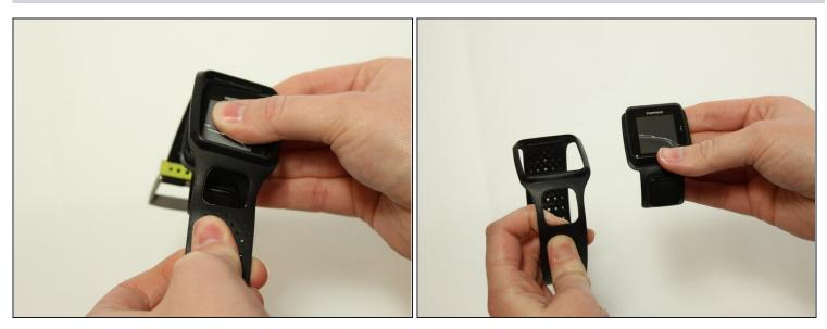
• Continue to lift up on the band until the screen of the watch becomes loose from the band.
