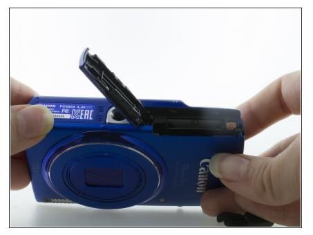
With the door open, locate the orange clip near the edge of the camera. This clip is holding the battery in place.
