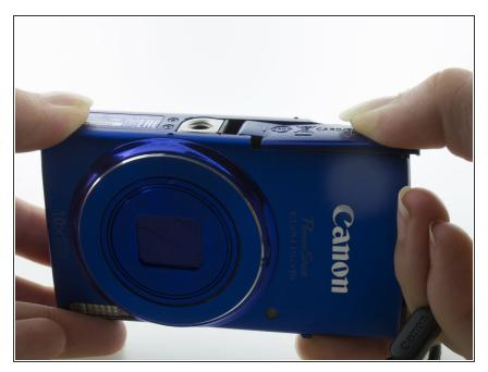
Press the door down with your thumb and slide to the right until you hear a click. This means the door has unlocked and will open.
