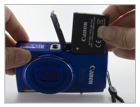
• The battery should pop out easily and you can simply remove the battery from its housing.
