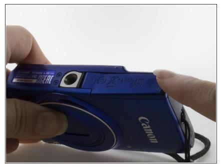
Locate the Battery door which is marked, "CARD/BATT OPEN"
