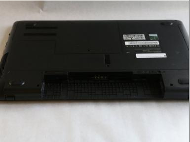
Completely remove the battery from the laptop.
