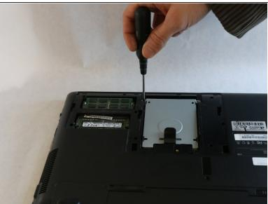
• Locate the gray hard drive cover, and remove the four corner 3.5mm screws.
