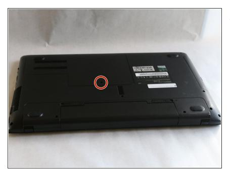
Remove the 4mm screw with a Phillips #0 screwdriver.
