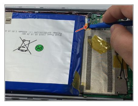
Free the battery from the motherboard by prying slightly with the opening tool.
