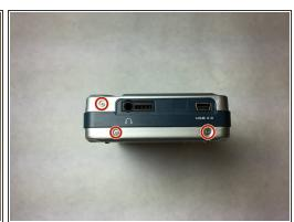
• Use a J0 screwdriver to remove the eight 3.5mm screws.
