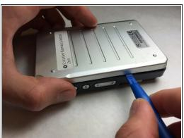
Use the plastic opening tool to open the top cover by carefully prying at each corner.
