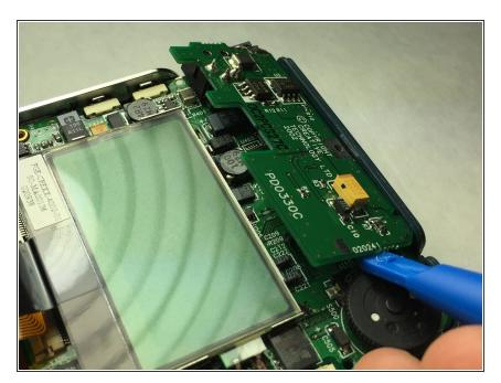
Using the plastic opening tool, gently pry up the other side of the auxiliary jack motherboard.
