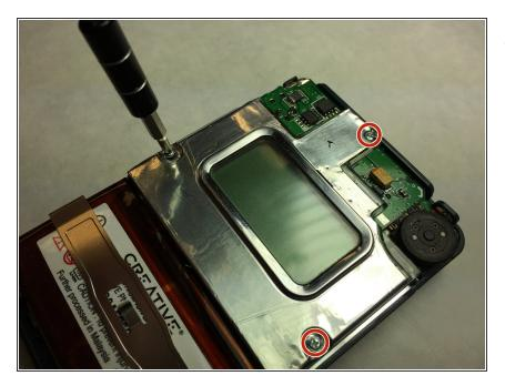
Once the front face is removed, remove the three 6.8mm J0 screws from the metal cover and remove it.
