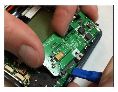
Using the plastic pulling tool, pull the plastic housing of the device out of the way in order to wiggle the the auxiliary jack motherboard free.
