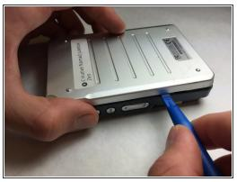
• Use the plastic opening tool to open the top cover by carefully prying at each corner.
