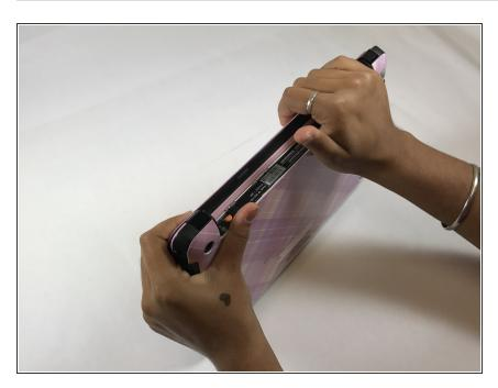
Remove the battery from the device.
