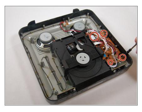
After removing the top of the device, locate the screws on the motherboard. Gently unscrew all four of the 3.5mm screws on the motherboard.
