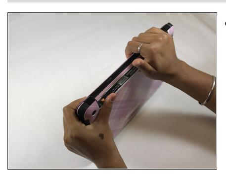
Remove the battery from the device.
