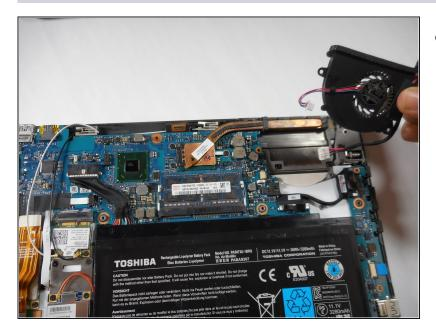
• Gently use you thumb and forefinger to lift and remove the fan.
