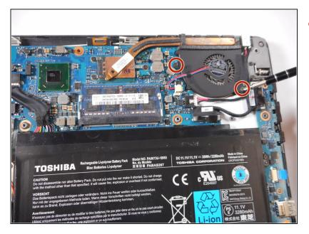
• Unscrew the two 5.4 mm screws with a PH1 screwdriver.
