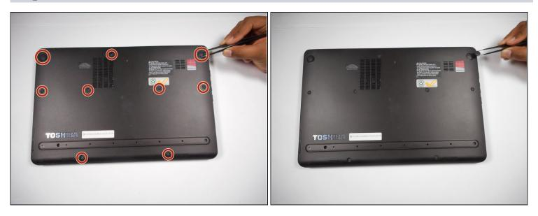
• Use <u>tweezers</u> to remove the 9 rubber grip pads on the back panel of the laptop.
