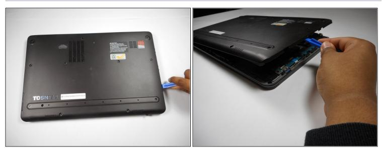
• Remove the back panel by inserting the plastic opening tool into the seam of the laptop, and pushing the opening tool downwards.
