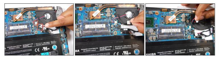
• Pull the cables away from the two connectors in the same direction as the individual wires are running.
