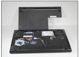
Remove the placeholder screws and pull off the backplate.
