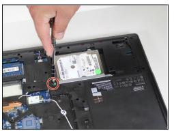
• Using your Phillips Screwdriver, remove the four screws around the hard drive.
