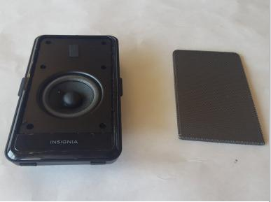
Once there is a big enough gap, insert the metal spudger and remove the tweezers. Move the spudger around the edge of the mesh to remove it.
