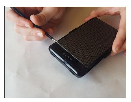
Use the tweezers to lift the corner of the mesh until a gap is created.
