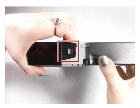
Lift the tabs located on each side of the device to free the front cover.
