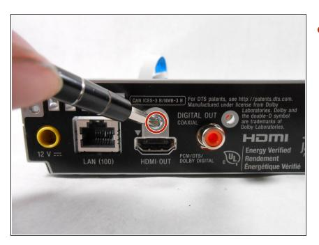
Unscrew 3mm Philips head HDMI screw from metal casing.
