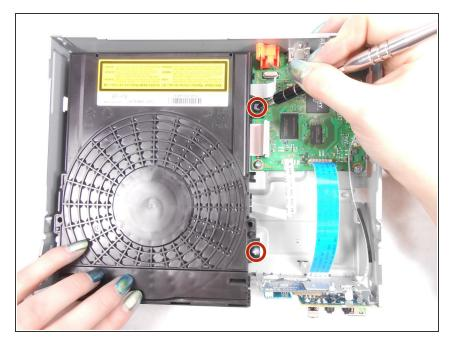
Unscrew the two 8mm Philips head screws securing the disc assembly to the main casing.
