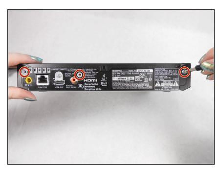
Remove the three 10mm Philips head screws on the back of the player.
