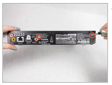
Remove the three 10mm Philips head screws on the back of the player.
