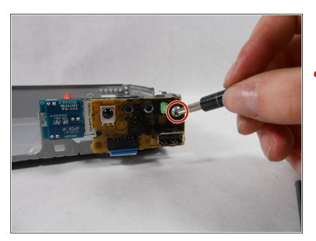
Unscrew the one 5mm Phillips head screw from the front of the device board.
