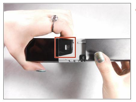
Lift the tabs located on each side of the device to free the front cover.
