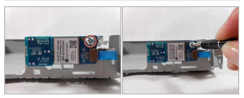
Remove 6mm Philips head screw from wifi board.
