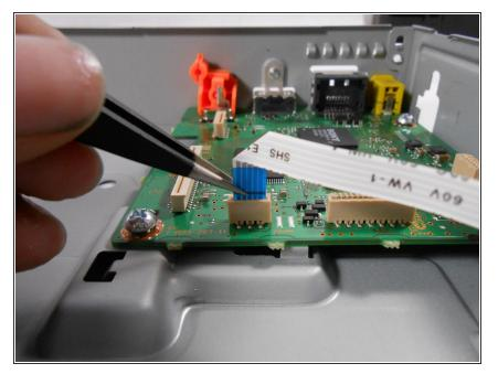
Remove the ribbon cable from motherboard using a pair of tweezers.
