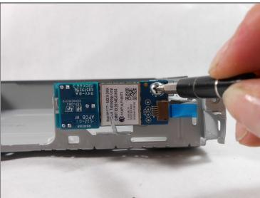
• Remove 6mm Philips head screw from wifi board.
