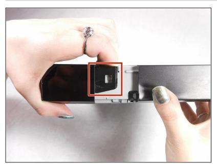
Lift the tabs located on each side of the device to free the front cover. Begin separating the two covers from metal casing.
