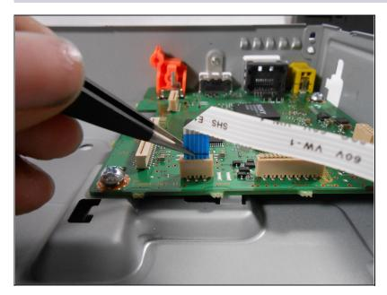
Remove the ribbon cable from motherboard using a pair of tweezers.
