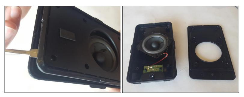
Once all seven 5mm screws are taken off use the metal spudger again to pry off the plastic casing from the speaker.
