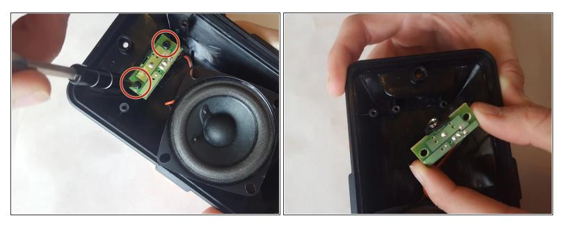
• To further take apart the speaker, there are also two 5mm screws on the green circuit board which keep the speaker and circuit board attached. Unscrew these with the size J0 JIS screwdriver.
