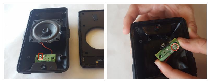
Follow <u>How To Solder and Desolder Connections</u> to desolder the circuit board's connection to the speaker cone.
