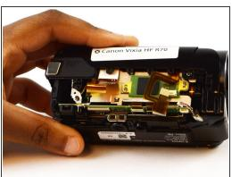
Disconnect the four ZIF connectors by grasping the connector firmly and pulling gently.
