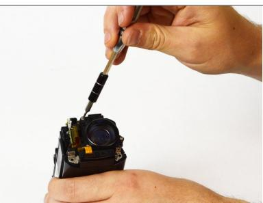
With the front of the camera facing you, locate and remove the three 5mm Phillips #00 screws that hold the lens in place.
