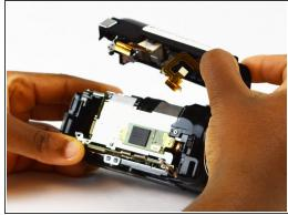
Pull the panel up and away until it is removed completely.
