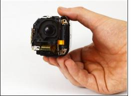
Grasp the plastic sides of the lens, and pull it away from the camera body to finish removing the lens.
