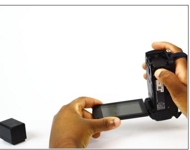
While holding down the latch, remove the battery by pulling it out of the device.
