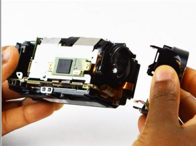
Pull the entire shutter away from the body of the camera to remove it.
