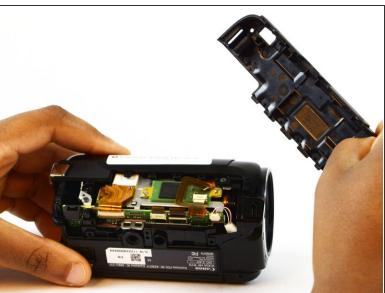
Gently remove the side panel by pushing it up from the bottom.
