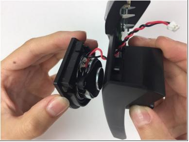
Once both speakers have been unclipped, gently pull the wire through the housing.
