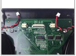
Disconnect the two white 2-pin JST connectors from the keypad/speaker circuit board by tugging gently until they release.
