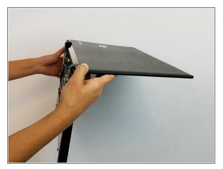
• Open the laptop at a right angle to make the later removal much easier.
