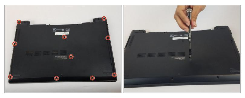
Unscrew the ten 6.5mm PH1 Phillips head screws that hold down the back cover.
