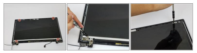
• Unscrew the four inner screws around the screen.
