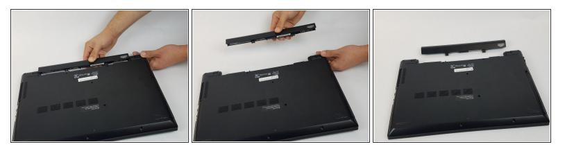
• Pull the battery out, keeping it flat and parallel to the laptop so that it slides out easily.
