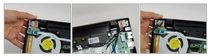
• Unscrew the four PH1 Phillips head screws on the hinges.
