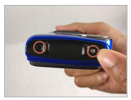
Unscrew two 4.0mm long hex head screws with a hex 1.3 screwdriver bit.
