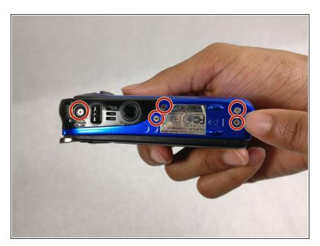
Unscrew five 4.0mm screws with a Phillips head 0 screwdriver
