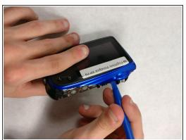
Pry the back plate off with a plastic opening tool
