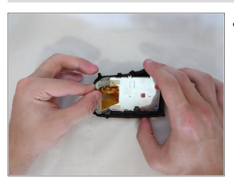
Use the plastic opening tool to gently lift the LCD screen up.
