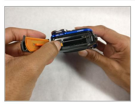
Pull the orange tab towards the hinge to release the battery.
