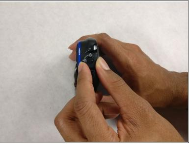
Push down on the center button and turn the dial on the side counterclockwise to open the battery compartment.
