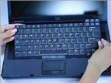
Remove the keyboard carefully now that it is detached, and use the pry tool to assist you in the removal of the keyboard.
