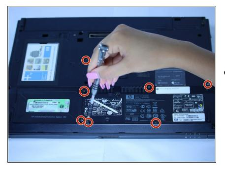
Use a J1 screwdriver to remove each screw on the bottom of the computer. This will allow for the
