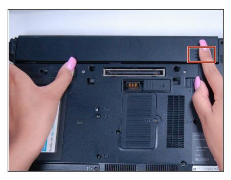
Slide up against the three lines the battery has.
